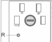
The initialization process starts automatically once power restored. For security reasons an electronic restart lock is activated. The initialization process can also be stared by pressing the reset button (R) (less than 2 seconds) on the key-operated switch.
