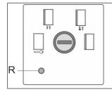
The operating modes LOCKED – AUTOMATIC – ONEWAY – CONTINUOUS can be set with the key-operated switch. The reset button (R) is also integrated in the key-operated switch, after pressing it the door control will be reinitialized.
